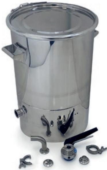
The Sampling Systems range of drums with a slanted base allow the drums to drain completely. The drums are finished to a mirror polish for easy cleaning. At the bottom of the slanted base is a ferrule for easy emptying.
