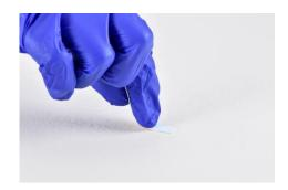
3) While holding the strip in your hand, wait 30 seconds to allow the color reaction to occur. Read out your results. The result is valid for five minutes after sampling. Results may be recorded by photograph.
